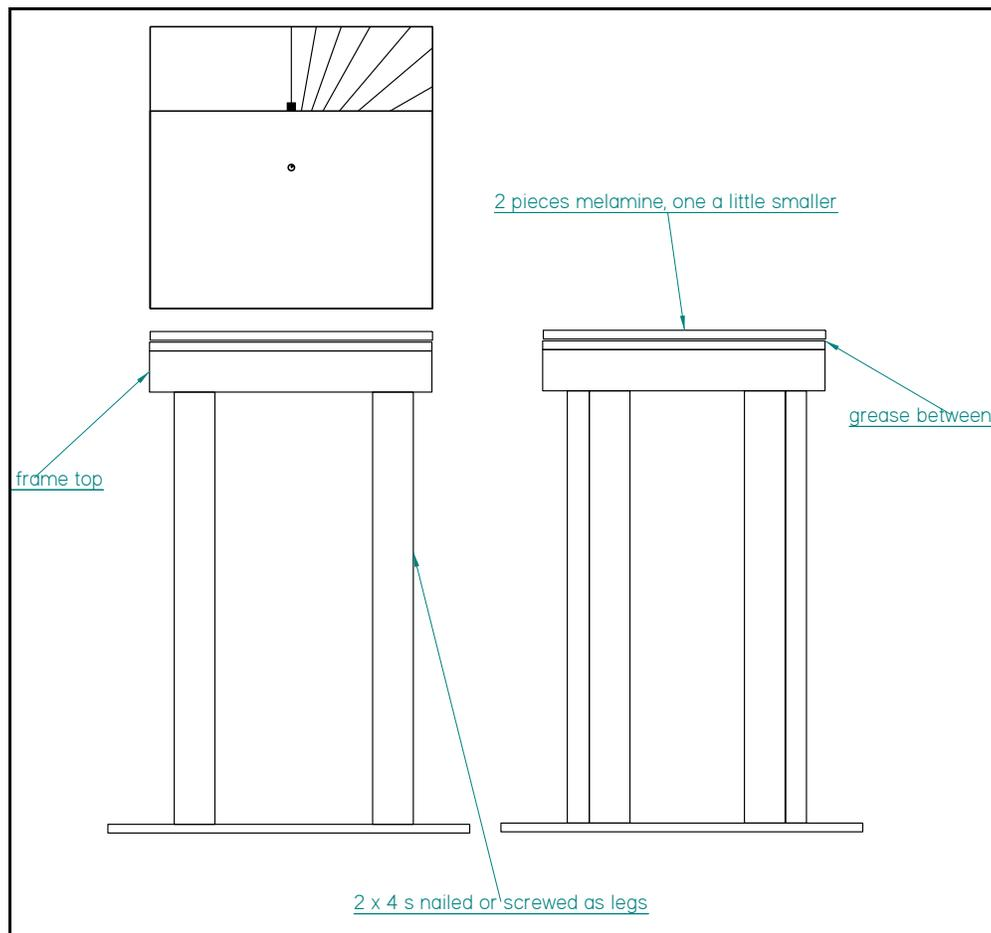
Draw lines from the rotation point out to the edge on  $\frac{1}{2}$  of the bottom plate (or you can do it all the way around.) It is best just to mark those angles that are actually used. I only mark a minimum of  $10^\circ$  because below this is hard to draw. Just measure between the  $10^\circ$  markings to get the  $5^\circ$  ones. A
