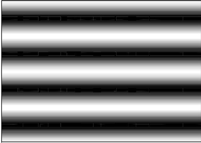
nents by  $k_x$  and  $k_y$ . The wavenumber is the number of wavelengths in a given distance. If the distance is defined to be the image width and the image height then the wavenumber are the same as the frequency.
