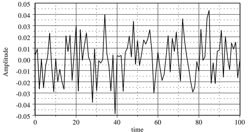
A third signal with a nearly flat spectrum is a swept sine wave. The details of using swept sine waves is too complex to get into here, but they are one of the most common and useful of all of the measurement signals and techniques.
