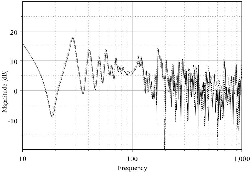
Figure 8-2 - A room calculation with a very small perturbation of the wave speed
