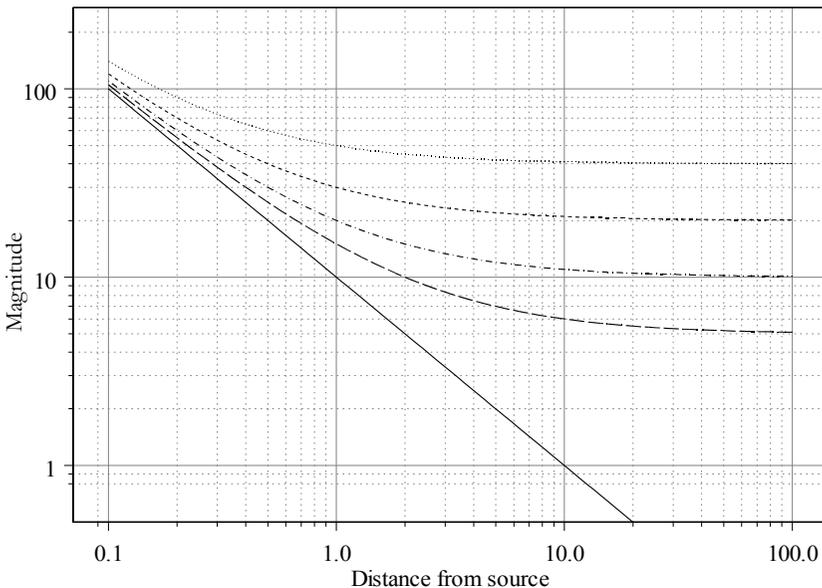
Figure 8-7 - Falloff of sound level in a reverberant field for several values of reverberation
