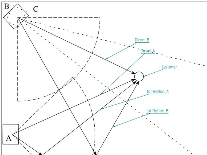
*Figure 8-8 - Room layout showing coverage of directive sources in two different configurations*
