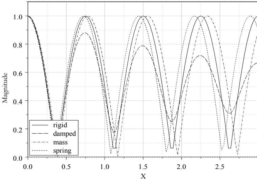
Figure 8-6 - modal functions for mode four with various wall impedances
