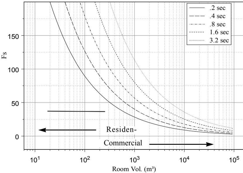
Figure 8-5 - Schroeder frequency versus room volume and reverberation time
