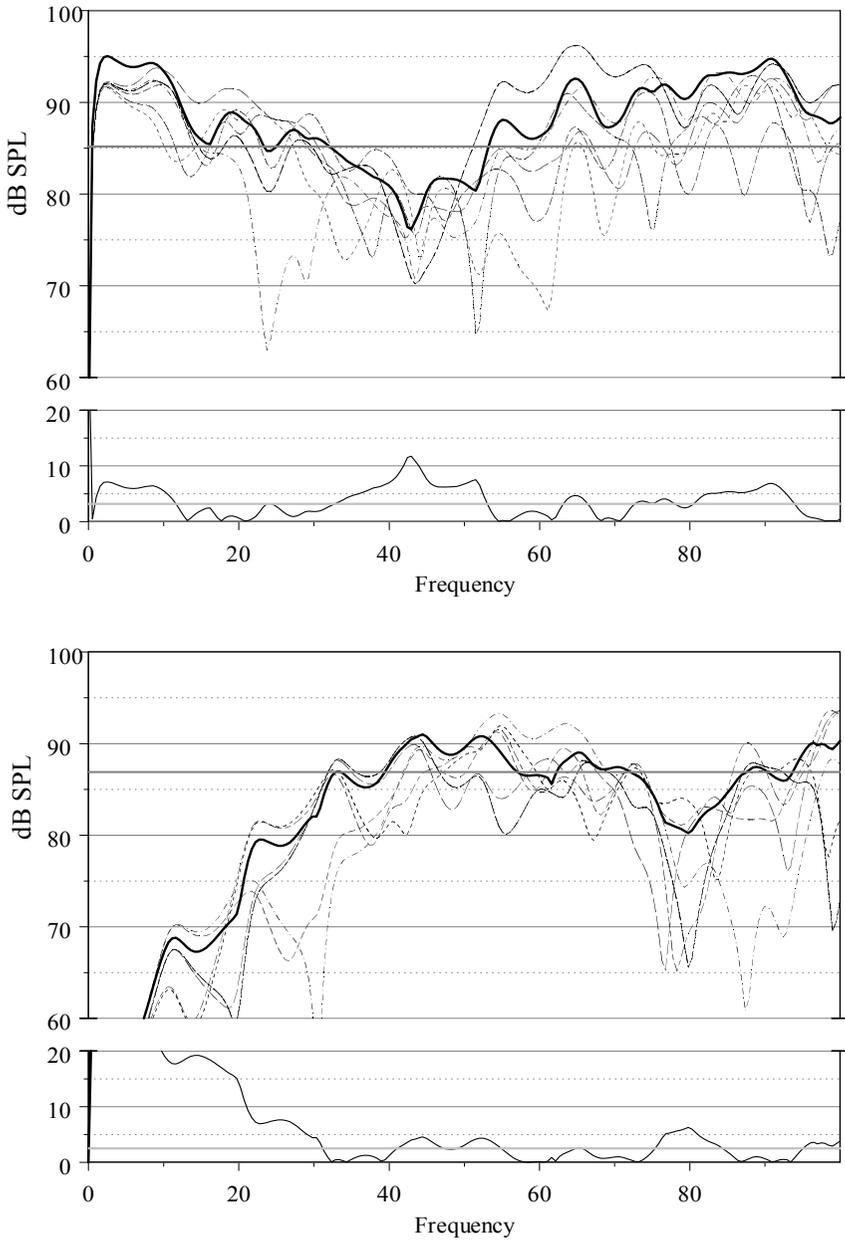
Figure 8-9 - Room responses for a monopole and a dipole
