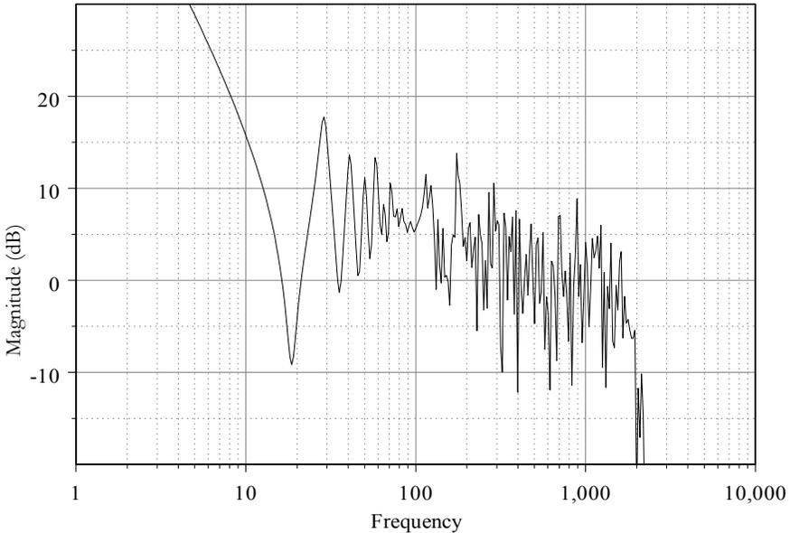
Figure 8-1 - Typical room response for a closed room with rigid walls
