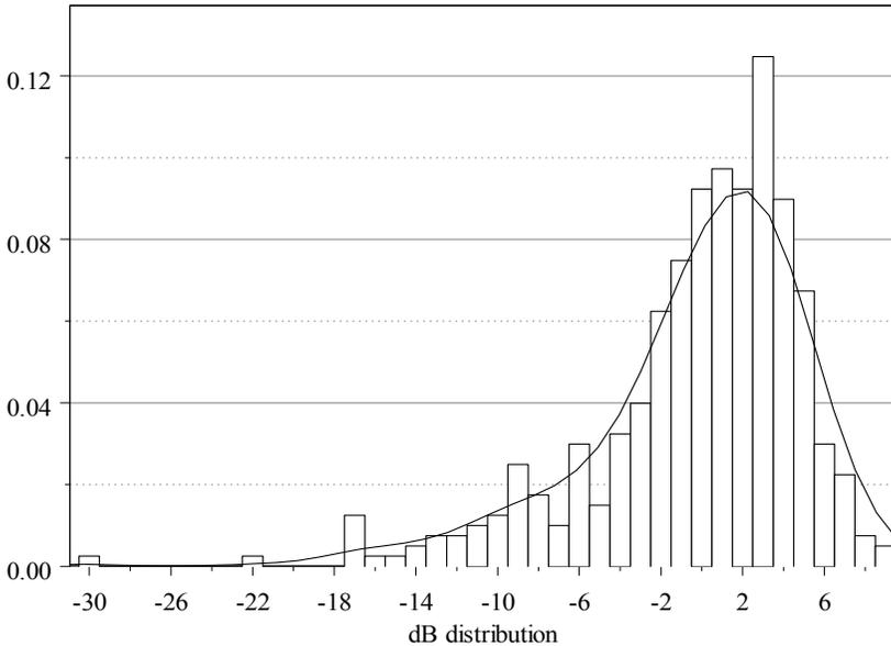
Figure 8-4 - The probability distribution in dB level for the pressure response in a room
