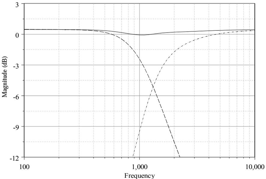
Figure 7-8 - The axial response of the large driver response
