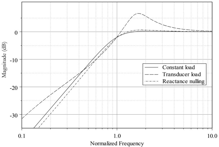
Figure 7-10 - The electrical response of a passive high pass filter with a constant load, a transducer load and a nulling circuit
