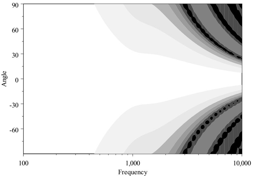
Figure 7-7 - Vertical and horizontal polar maps for directional two way system
