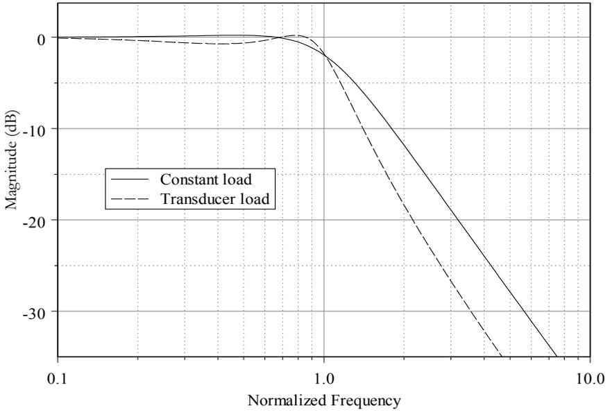
Figure 7-9 - The electrical response of a passive low pass filter loaded by a transducer impedance
