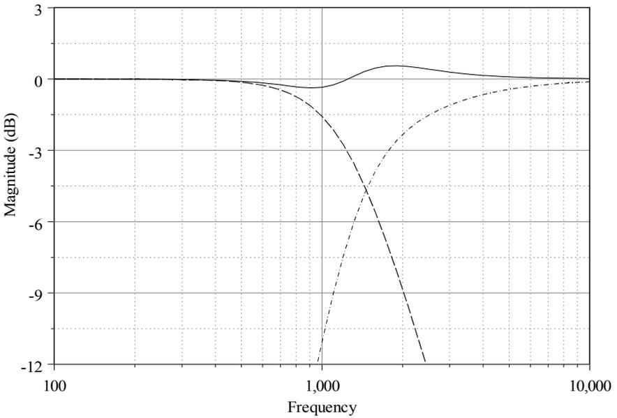
Figure 7-5 - Axial frequency response for typical two way loudspeaker
