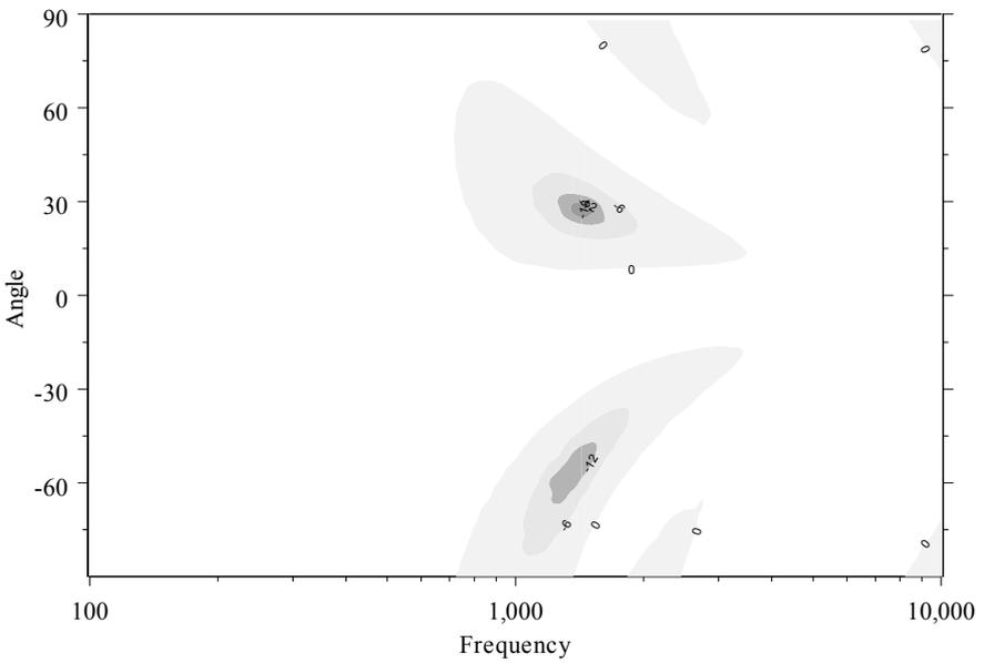
Figure 7-6 - Polar response maps for a typical two way loudspeaker system
