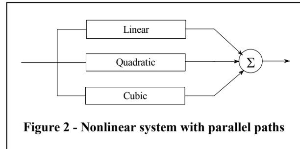
**Figure 2 - Nonlinear system with parallel paths**
