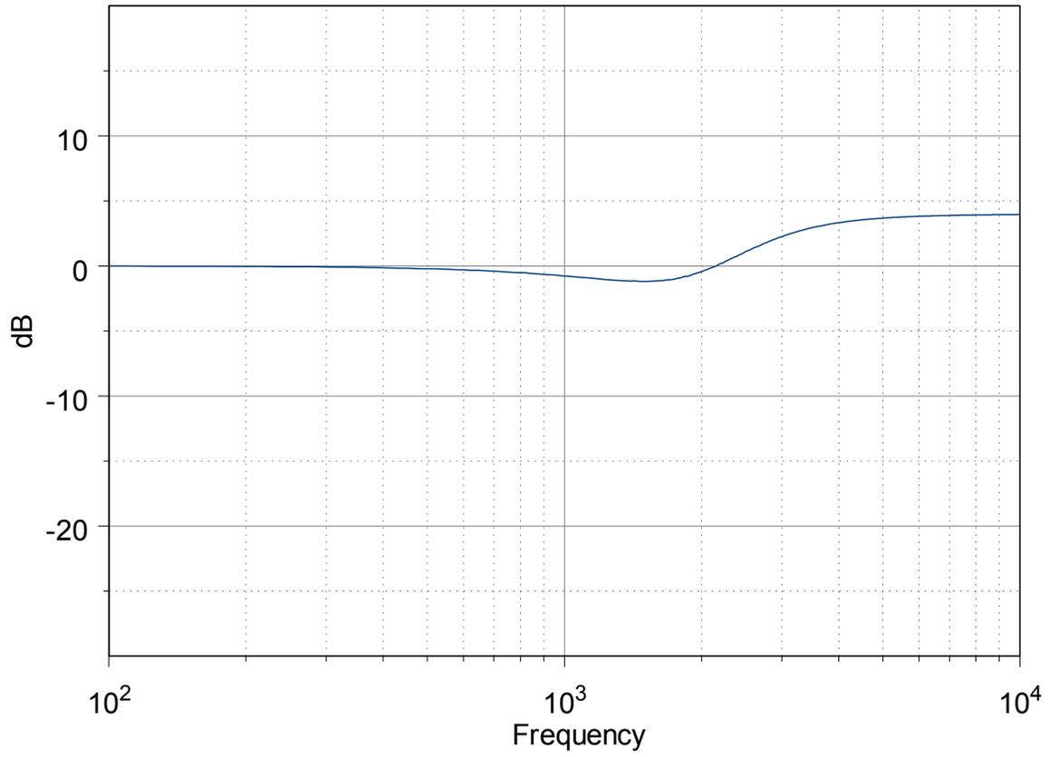
Figure 1 - Filter response for zero delay + 4 dB stimulus
