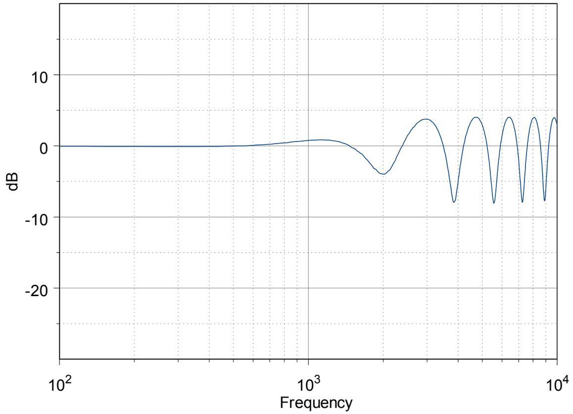
Figure 2 - Filter response for delay = .6 ms, + 4 dB stimulus.
